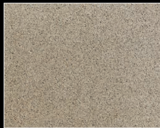
Stanford Sand FM Thermal Emittance 0.94 SRI 48 Solar Reflectance 0.39
