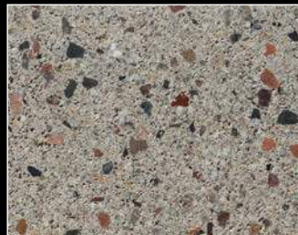
Delta White FM w/AZ Del Mar Agg Grind Thermal Emittance 0.90 SRI 40 Solar Reflectance 0.36
