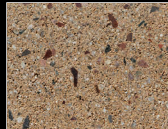
Delta Yellow FM w/AZ Del Mar Agg Grind Thermal Emittance 0.90 SRI 41 Solar Reflectance 0.37
