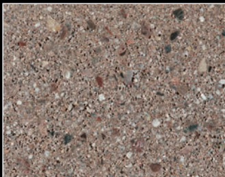
Delta Beige FM w/AZ Del Mar Agg Grind Thermal Emittance 0.89 SRI 30 Solar Reflectance 0.29
