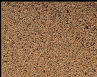
Port Yellow FM Thermal Emittance 0.92 SRI 44 Solar Reflectance 0.39
